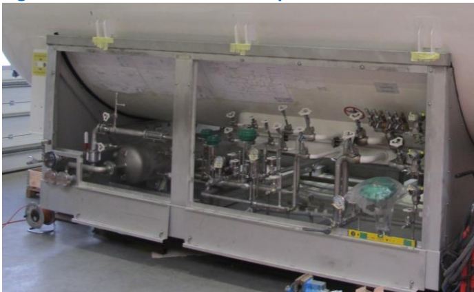
Figure 14: LNG tank connection space
