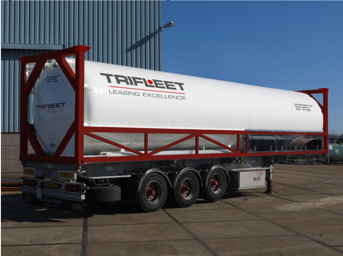
Figure 1: Standard 40' – 46000L 7/10 barg UN Portable T75 / ADR R14,3BN LNG tank.
